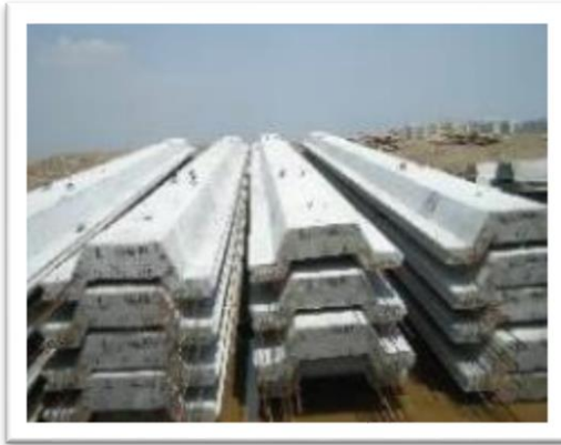
BETON PENAHAN TANAH
